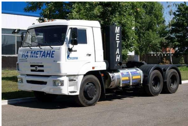
Figure 4. Truck Tractor KAMAZ-65116-34 on LNG with kriotank
