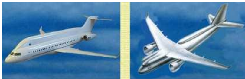
Figure 7. Aircraft TU-334K, Tu-330 K with LNG engines
