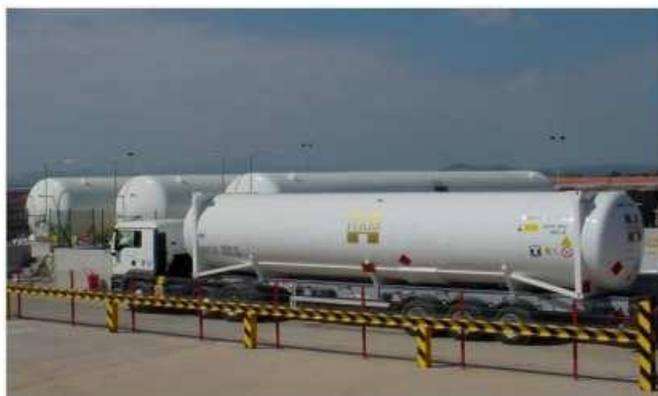
Figure. 3. Intermodal container for LNG (United States)
