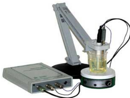
Fig. 1. The set for the measurements of the heavy metals in the laboratory and field conditions.
