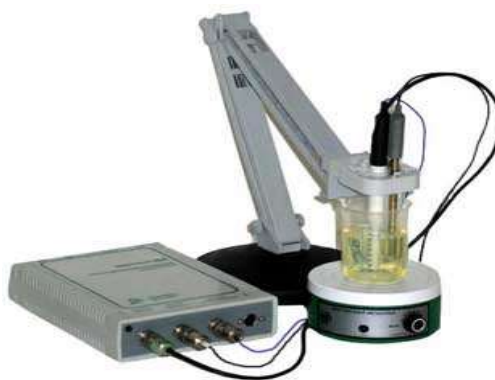
Fig. 1. The set for the measurements of the heavy metals in the laboratory and field conditions.
