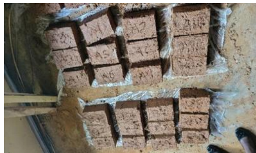
Figure 2. Shows the samples of bricks with varying percentages of pseudo stem fibre
